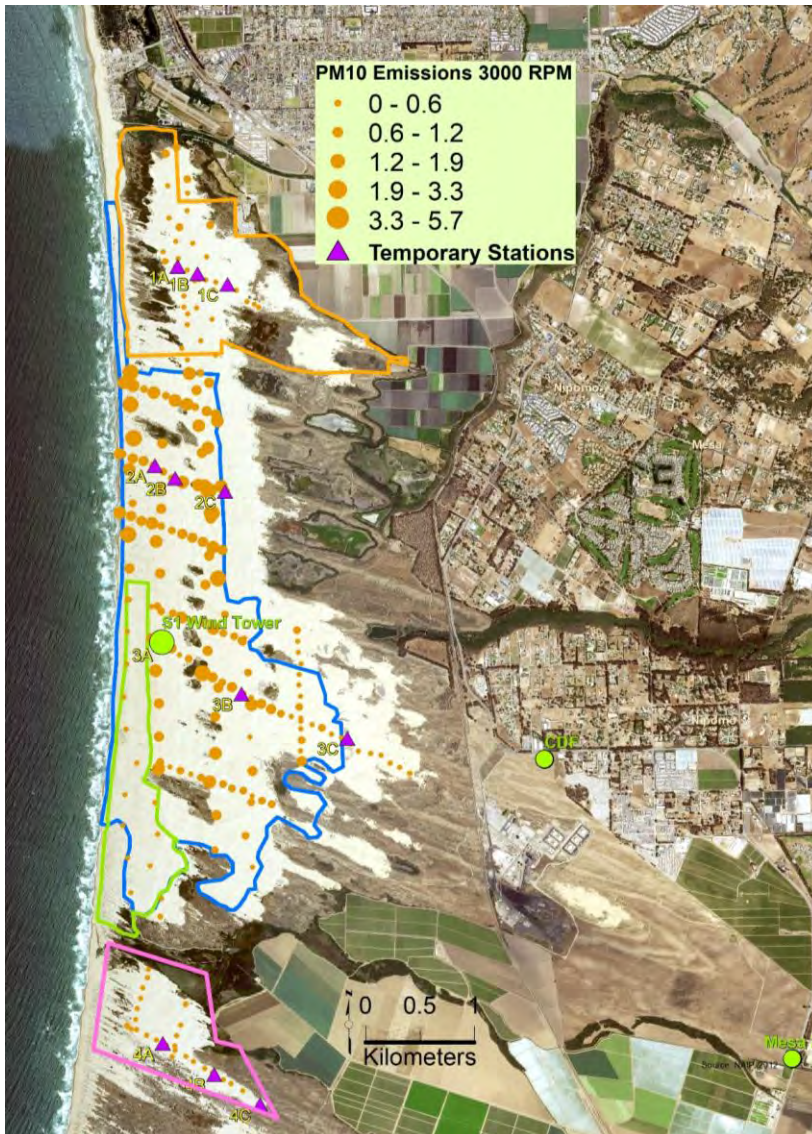
549 Figure 5. Spatial distribution of PI-SWERL measured PM_{10} emissions ( mg of PM_{10} m^{-2} s^{-1} ) at 3000 RPM, 550 which is equivalent to u_* = 0.53 m s^{-1} .
