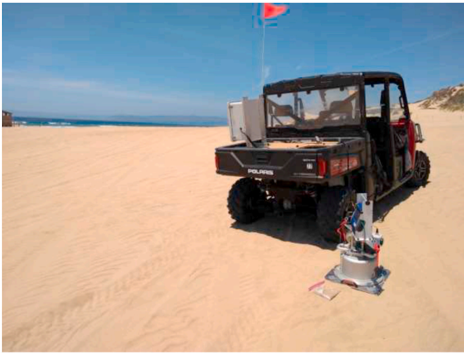
Fig. 2. The PI-SWERL at a test location in the riding area of the ODSVRA.
