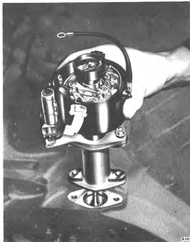
Fig. E55 Method of fitting distributor
