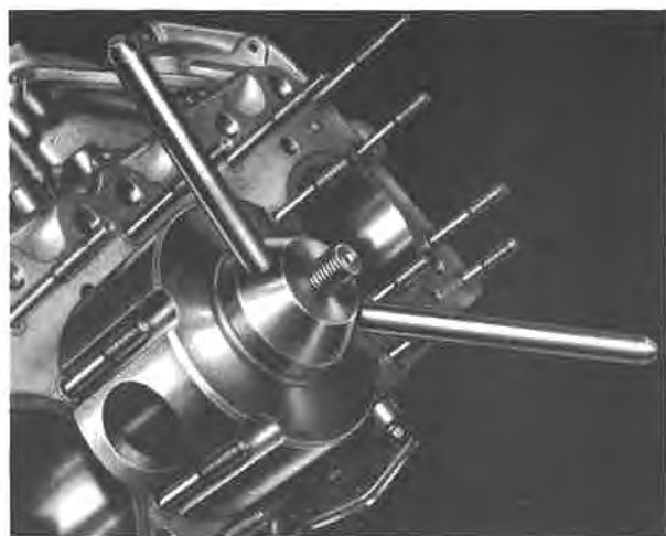
Fig. E16 Method of removing cylinder liner using tool No. RH.7095
