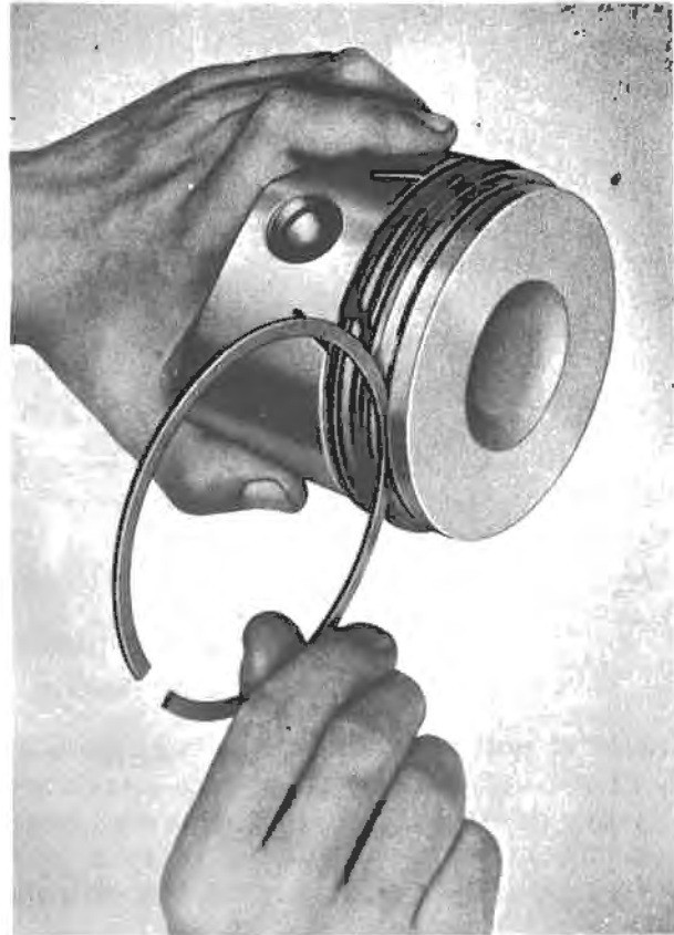
Fig. 41 Checking piston ring clearance
