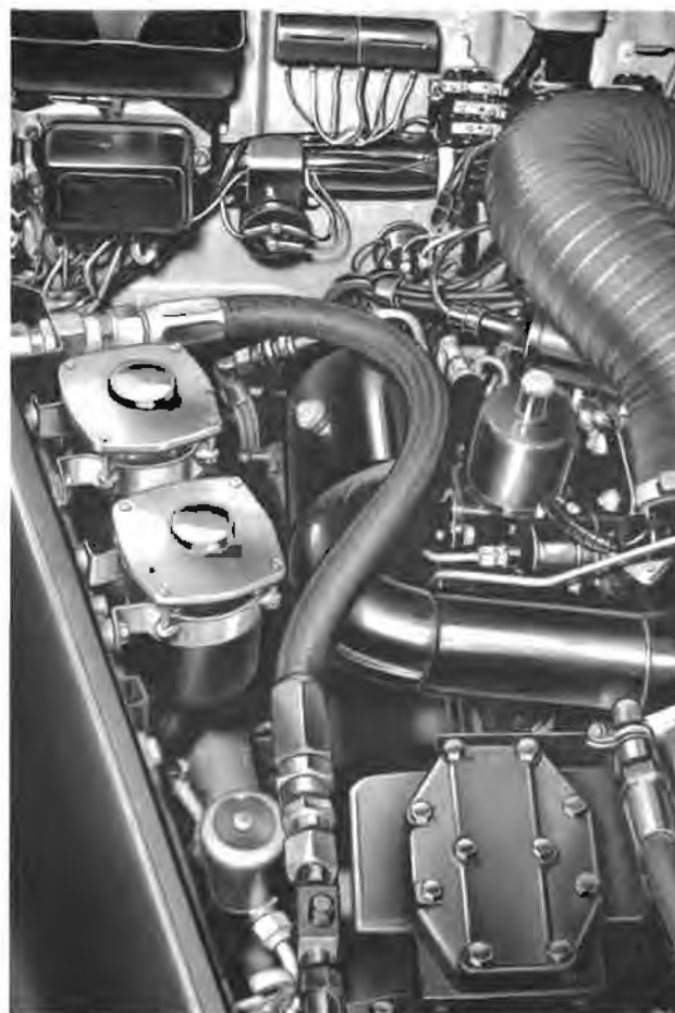
Fig. 16 Compressor and Refrigerant Lines
