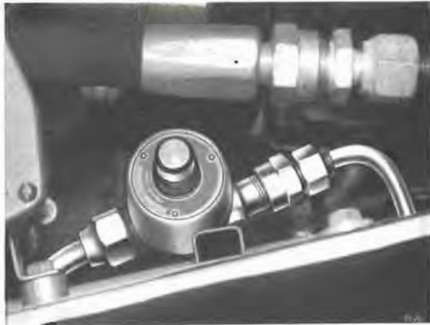
Fig. 15 Flow control valve
