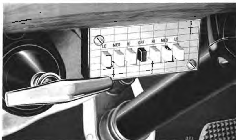
Fig. 5 Blower Motor Control Panel
