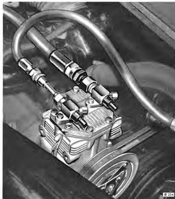
Fig. 12 York Compressor in Position
