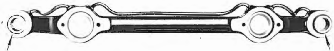
Fig.4. Idler cross beam - arrows show where burrs should be removed.
