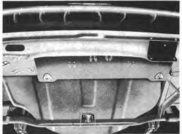
Fig.1. View showing slot and baffle plate in position.
