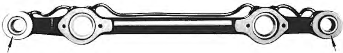
Fig.4. Idler cross beam - arrows show where burrs should be removed.
