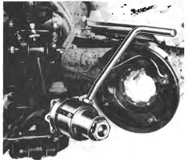
Fig. 2. Cutting tool assembled in readiness for cutting radius.
