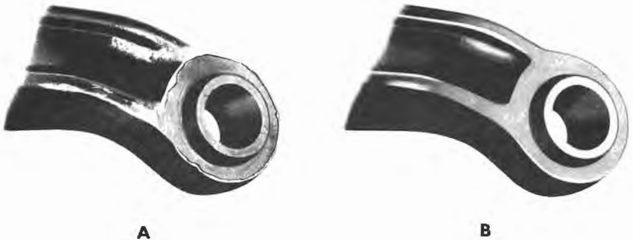
Fig.3. Side steering lever showing 'A' before and 'B' after burrs have been removed.
