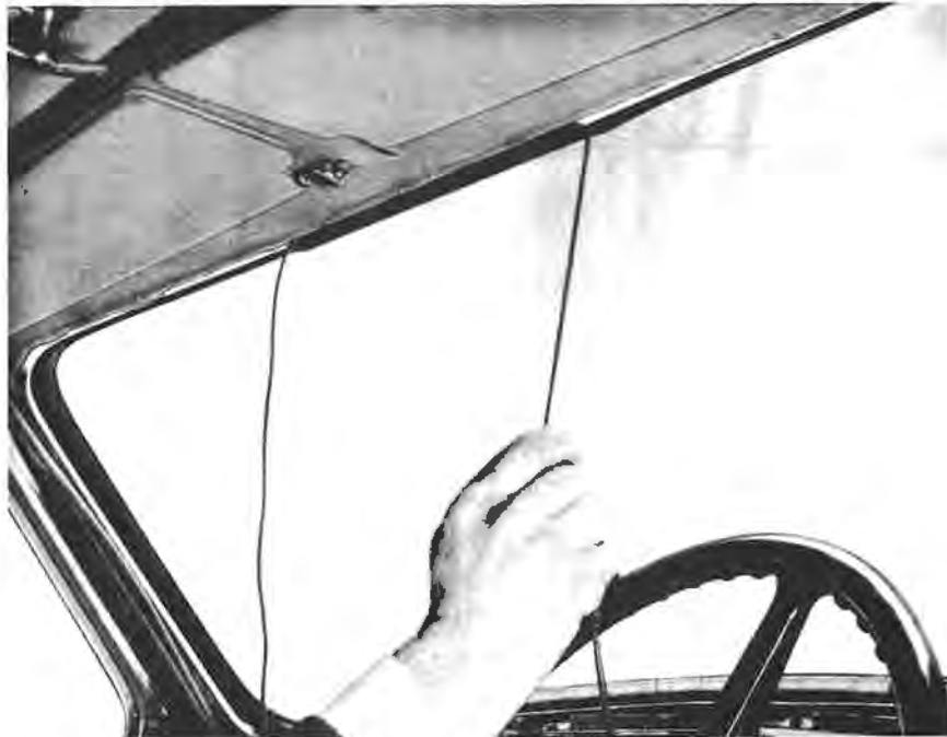
Fig. 3. View of windscreen showing process of drawing seal over retaining angle.
