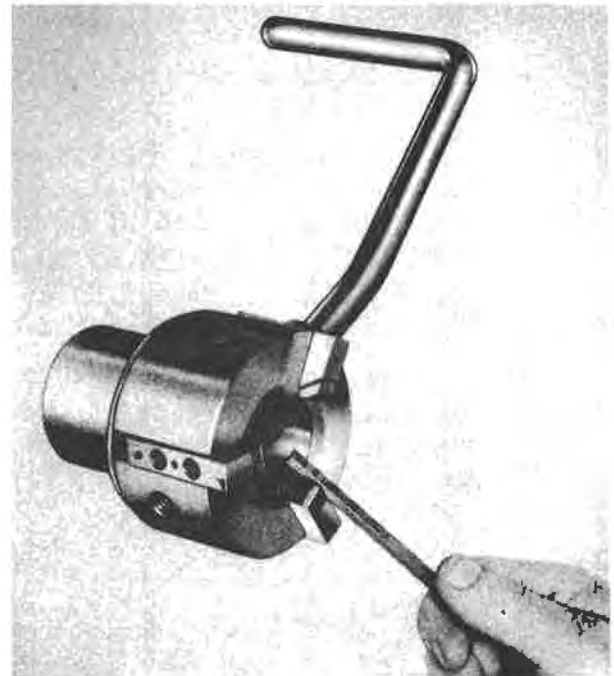
Fig. 4. Method of sharpening cutters.
