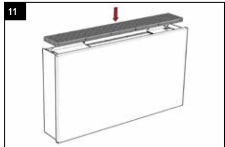
Place the grill ⚠ The direction of the airflow is determined by the shape of the fins of the grille.
