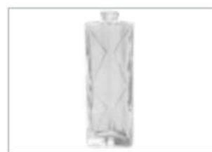
Hard glas (Boheems glas): \text{K}_2\text{O} vervangt \text{Na}_2\text{O}
