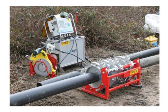
The ODS-Track machines fulfill the related CE Directives and the following ISO Specifications: 12176-1-3-4 for TWIN-S & DYNAMIC-S; 12176-2 and ISO/TR 13950 for TWIN-S.
