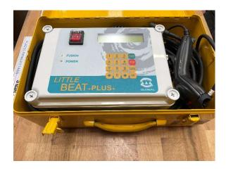
Super handy little electrofusion computer. Fully integrated in steel case. Suitable for welding fittings up to diameters 110 mm and some brands up to 160 mm.
