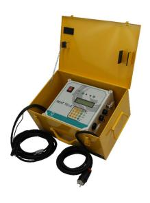
The electro welding computer BEAT MV2 was specially designed for the installer, for the electro welding of PE fittings for pipe with range up to 400mm and for HDPE. The BEAT MV receives the relevant data by manual input of voltage and time, or using barcode scanner.
