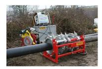
This ODS machine is the most compact butt welding equipment on the market for butt welding up to and including 630 mm.
