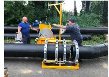
*These machines are also equipped with the traceability system. Can be controlled by both Smartbox and Polycontrol.*
