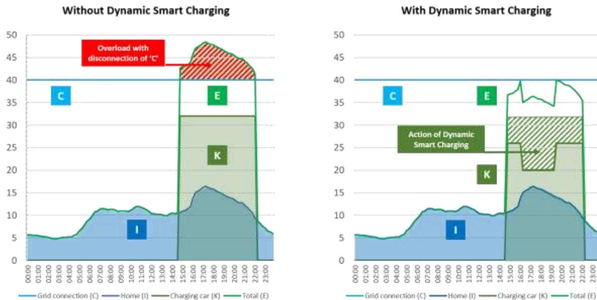
Figure 2: Influence of Dynamic Smart Charging on the maximum capacity of the electrical home connection
