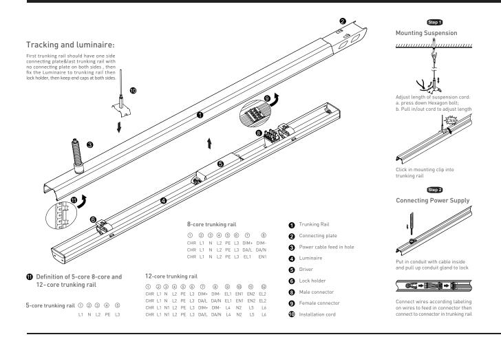
Connecting Trunking Rail Both trunking rails should keep in perfect position then push to click
