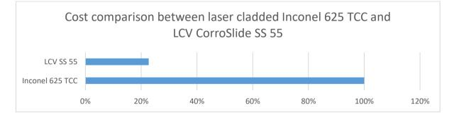
The SS 55 material is a significant cost saving alternative and can be applied at elevated temperature. Hardness is with 59HRC not in the same 60+HRC category as an Inconel 625 TCC but it concerns a mono-alloy which offers good wear resistance to both coarse and fine gritted abrasives. Corrosion resistance is based on the martensitic high chromium base material and can suit a wide range of applications.
