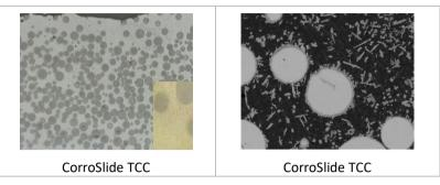
This results on average in **improved wear resistance**. Lifetime prediction is subject to service condition but on lab scale, laser cladded TCC coatings perform on average up to 4 times (4X) better than sprayed hard metallic overlays and conventionally welded hard-facing.
