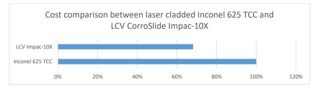
The IMPAC-10X material is an interesting material when both wear resistance and toughness is required. The material is less suited for high-temp applications or corrosive service conditions. It is a speciality material which represents still a cost saving compared to the Inconel 625 TCC cladding and for selected types of applications it can yield significant TCO savings.
