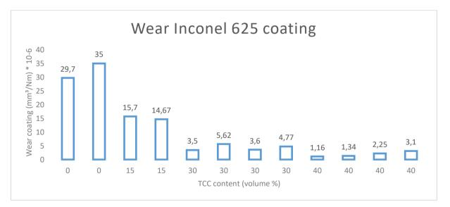
For many applications, Inconel 625 TCC is a <u>proven performer</u> as it benefits from the Inconel 625 reputation and combines this with the ideal carbide integration which yields enhanced abrasion resistance. Caution applies for the abrasive media as very fine granulate (P50 and less) can erode the softer Inconel matrix.
