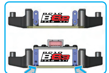
New holes added to chassis for servo mount
