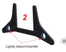
2. Use a hobby knife, deburr and slightly chamfer the underside of the 3008 tweak plate where the damper cup will be placed (large 8mm holes). While this is not mandatory, it will help the
