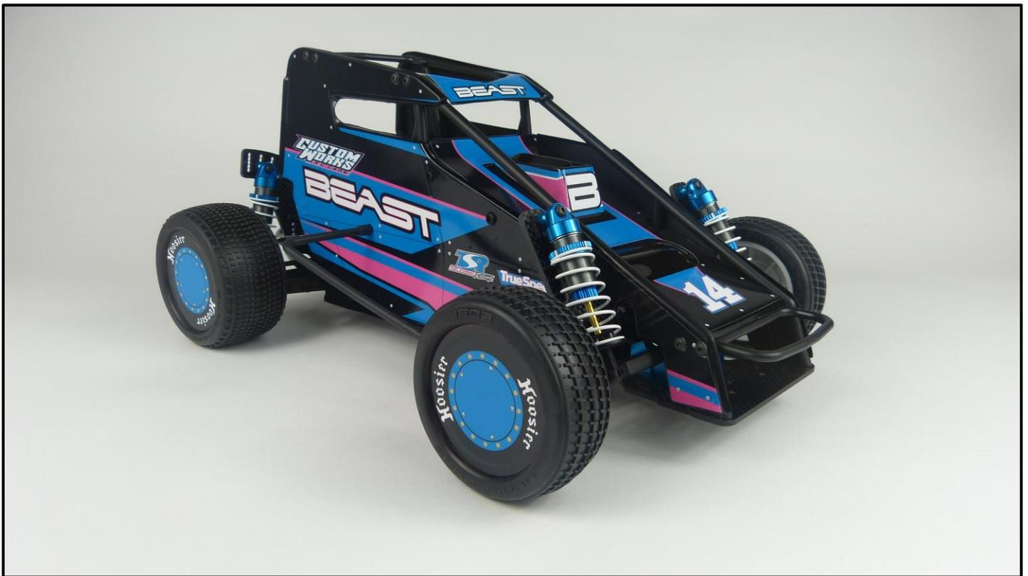
*Basic set-up – use the included turnbuckle wrench to fine tune the steering and camber links. Begin with a slight amount of toe-out on the front wheels. Make sure the servo saver is centered when the wheels are centered. Adjust the camber links so that the top of all 4 tires lean to the left slightly (1 degree.)*
