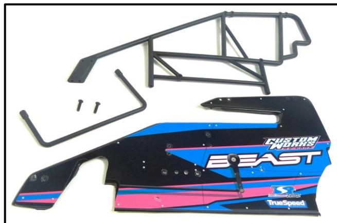
2. Place the body side panel on the cage side and use the two screws in the positions shown to mount the nerf bar.
