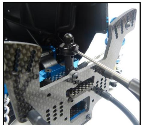
13. Position the tail tank on the body post and install the body clip.
