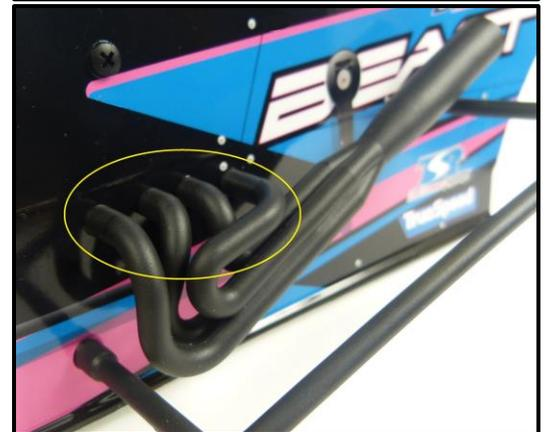
9. Using the remaining 6pcs of 5362 M3x12 screws and 2pcs of 9900 nylon screws & nuts (like used in step 4), fasten the right side of the cage to the rest of the assembly from the previous steps.
