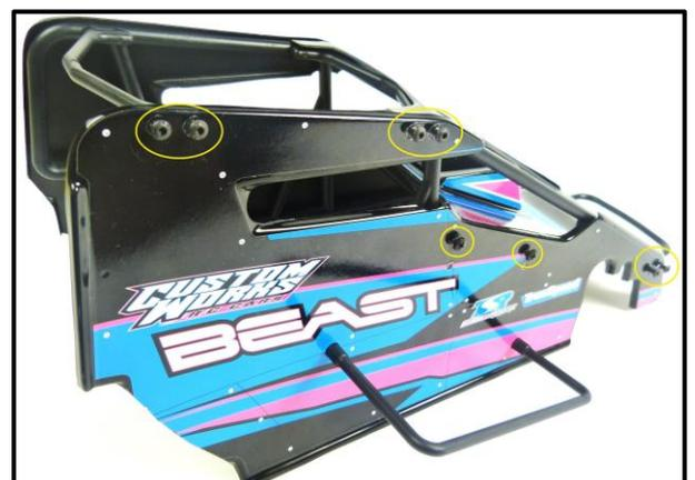
10. Locate the 8pcs of 5348 M3x8 Flat Head screws and use them to fasten the cage assembly to the chassis as shown.
