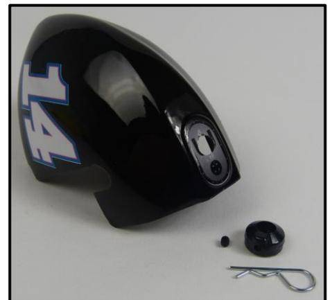
12. Install the set screw into the body post collar and snug the set screw into place on the body post in the position shown. Be careful not to overtighten the set screw.
