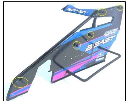
5. Install the halo bars and front bumper with the steel screws. Mount the left side of the hood using the nylon screws & nuts.
