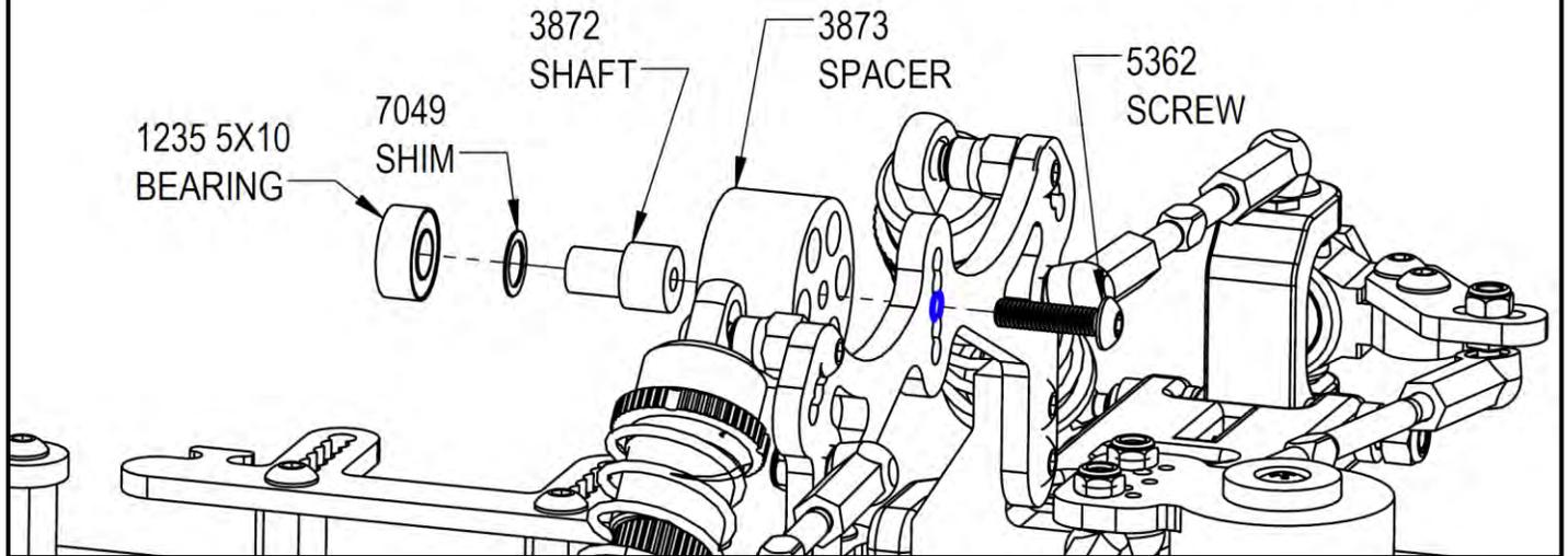
**\*ATTACH REAR SPACER TO FRONT OF REAR SHOCK TOWER\***
