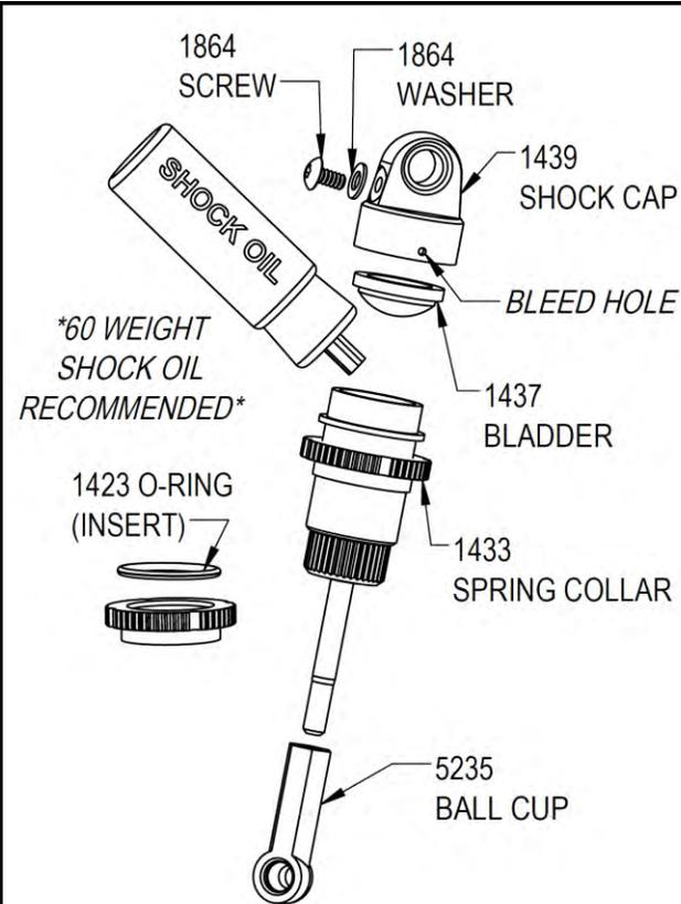
The diagram shows the shock assembly components and the process of filling it with oil. The components are labeled as follows:
