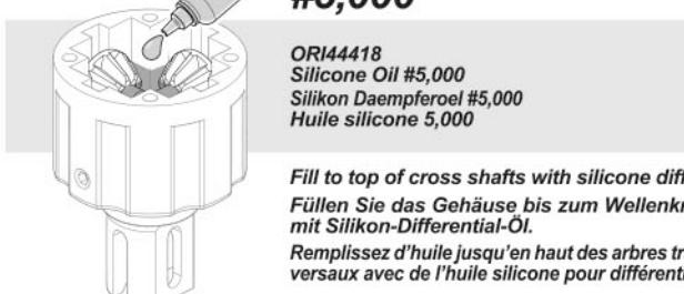
Fill to top of cross shafts with silicone diff oil.
