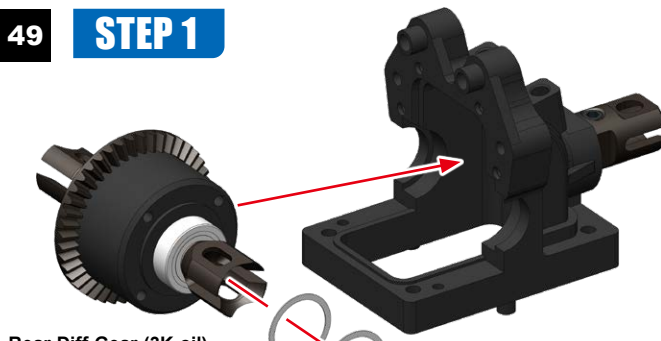
Rear Diff Gear (3K oil) リアデフギヤ (#3000 オイル)
