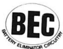
The radio contained in the box with this logo is the BEC type. As shown in step 37 on page 18, the radio does not use the regulator (30), also the wiring for the switch is not required. When using this type of radio, fix the BEC connector as illustrated below.
