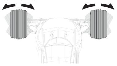
Perform a control test with the vehicle wheels off the ground. If the wheels rotate after the vehicle is powered ON, adjust the Throttle Trim until they stop. To make the wheels move forward, pull the trigger. To reverse them, wait for the wheels to stop, then push the trigger. When moving forward, the wheels should maintain a straight line without any steering wheel input. If not, adjust the Steering Trim, so the wheels maintain a straight line without having to turn the steering wheel.
