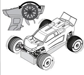
**4.** Start driving slowly, and, if the vehicle does not go straight, adjust the steering trim dial on the transmitter.
