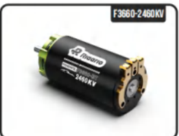
F3660-2460KV WATERPROOF BRUSHLESS MOTOR, SUPPORT BATTERY: 6S, MAX.VOLTAGE: 24V, MAX.CURRENT: 56A, 1350W, MAX.RPM: 60K, SHAFT DIA.: 5MM
