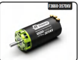
F3660-3570KV WATERPROOF BRUSHLESS MOTOR, SUPPORT BATTERY: 4S, MAX.VOLTAGE: 16.8V, MAX.CURRENT: 80A, 1350W, MAX.RPM: 60K, SHAFT DIA.: 5MM
