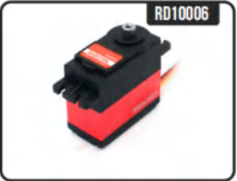
23KG STEERING SERVO, METAL GEAR, 120-DEGREE ANGLE, OPERATING SPEED(6V/8.4V): 0.18/0.16SEC, TORQUE(6V/8.4V): 19.2/23KG.CM. WEIGHT: 62G
