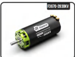
F3670-2830KV WATERPROOF BRUSHLESS MOTOR, SUPPORT BATTERY: 4S, MAX.VOLTAGE: 21V, MAX.CURRENT: 85A, 1800W, MAX.RPM: 60K, SHAFT DIA.: 5MM
