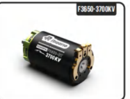
F3650-3700KV WATERPROOF BRUSHLESS MOTOR, SUPPORT BATTERY: 4S, MAX.VOLTAGE: 16V, MAX.CURRENT: 56A, 900W, MAX.RPM: 60K, SHAFT DIA.: 3.175MM
