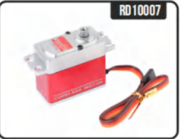
46KG STEERING SERVO, METAL GEAR, 180-DEGREE ANGLE, OPERATING SPEED(6V/7.4V): 0.13/0.11SEC, TORQUE(6V/7.4V): 38.6/46.8KG.CM. WEIGHT: 72G
