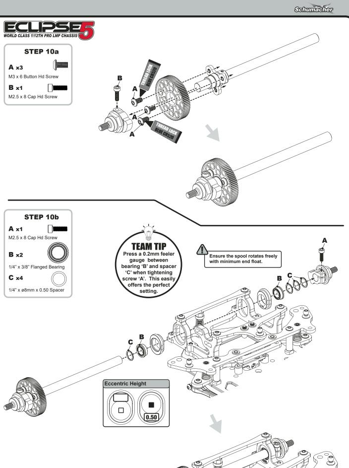
The eccentrics are used to adjust the ride height. There are 8 different eccentrics, 7 of which can be flipped to give a total of 15 options. See page 17 to choose an appropriate one for your tyre size.
