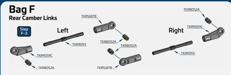
Build Tip: Use some grease of Chapstick to make assembly and future adjustments easier.
