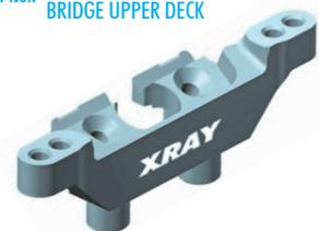
Alu front roll-center holder increases strength, reliability and makes the handling more precise and more forgiving.
