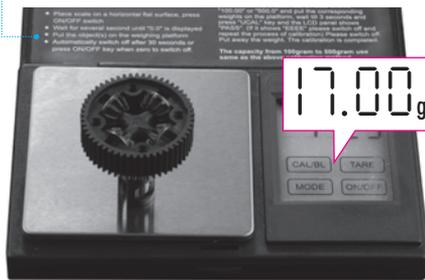
1 Put the diff (without oil) on the scale and check the weight (approximately 17.00g)
