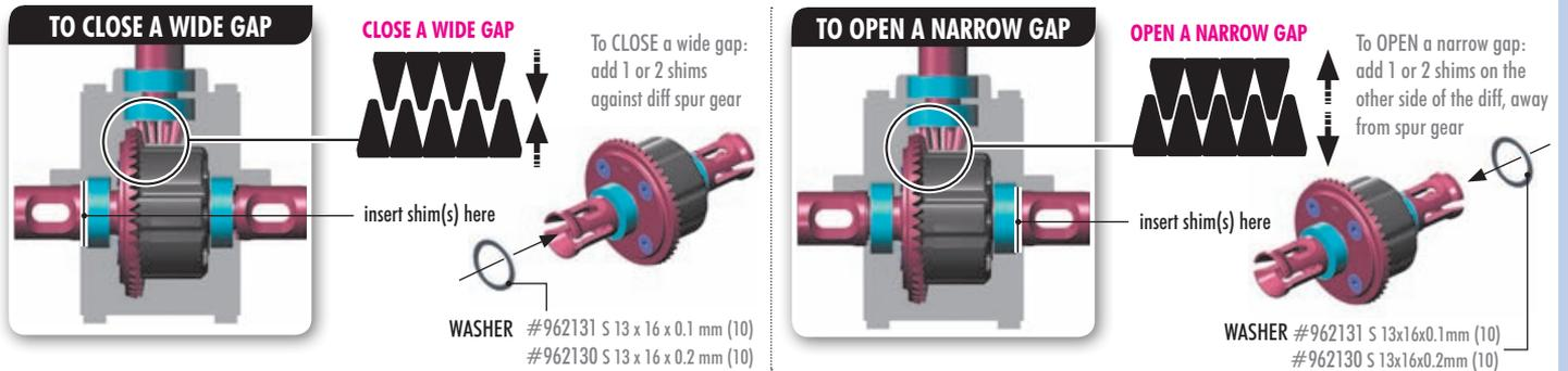
**CHECK GEAR MESH AND DIFF PLAY ONLY AFTER THE ENTIRE GEARBOX IS MOUNTED TOGETHER WITH THE SUSPENSION HOLDERS ON THE CHASSIS. ALL PARTS ARE DESIGNED TO HAVE CERTAIN PLAY AND IT IS ALL DESIGNED BY PURPOSE.**
