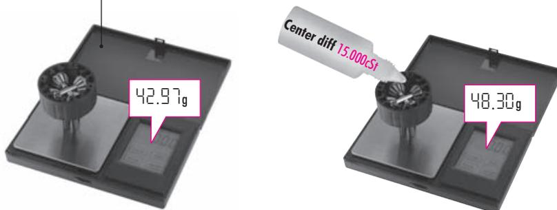
1. Put the diff (without oil) on the scale and check the weight (approximately 42.97g).
