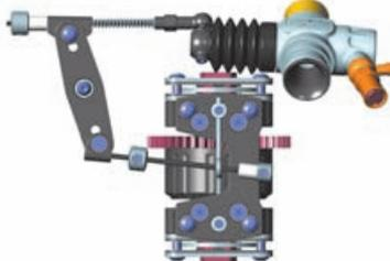
Adjust the servo-horn mounting position for the carburetor to open fully. Change the pivot mounting position on the servo horn in case the carburetor is not opening fully or if it is opening excessively. Or if available on the transmitter, adjust the throttle high end point.
