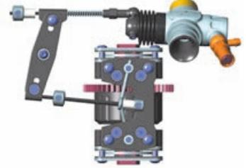
Adjust the adjustable collars so the brakes work smoothly. If the brakes apply too much or not enough, adjust the adjustable collars accordingly. Or if available on the transmitter, adjust the brake endpoint. To tighten brakes, turn collar to thread brake rod INTO pivot. To loosen brakes, turn collar to thread brake rod OUT of pivot.
