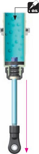
Extend the shock shaft completely. Fill the shock body with the shock oil. For the FRONT shocks (short) use 550cSt oil. For the REAR shocks (long) use 450cSt oil.
