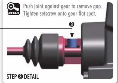
Push joint against gear to remove gap. Tighten setscrew onto gear flat spot.
