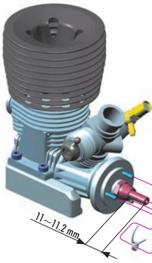
**!** Note the orientation of the clutch shoes. The short side of spring must be in the groove of the flywheel nut.
