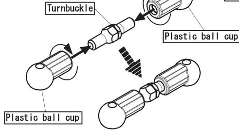
Assemble the tie-rod by attaching a plastic ball cup to both ends of the turnbuckle.
