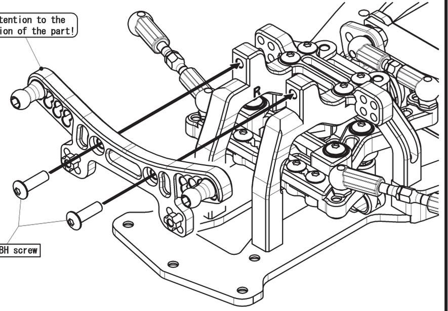
**Installing on rear shock tower**
