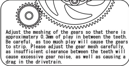
Adjust the meshing of the gears so that there is approximately 0.3mm of play in between the teeth. Be careful, as too much play will cause the gears to strip. Please adjust the gear mesh carefully, as insufficient clearance between the teeth will cause excessive gear noise, as well as causing a drag in the drivetrain.
