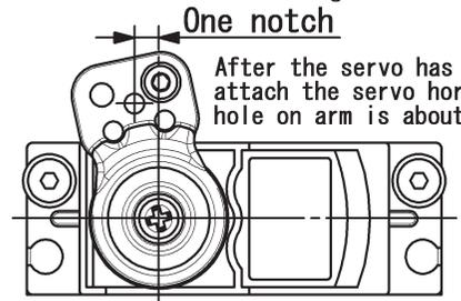
Make sure that the ends of the servo horn spring do not catch on the edges of the servo horn ring.
