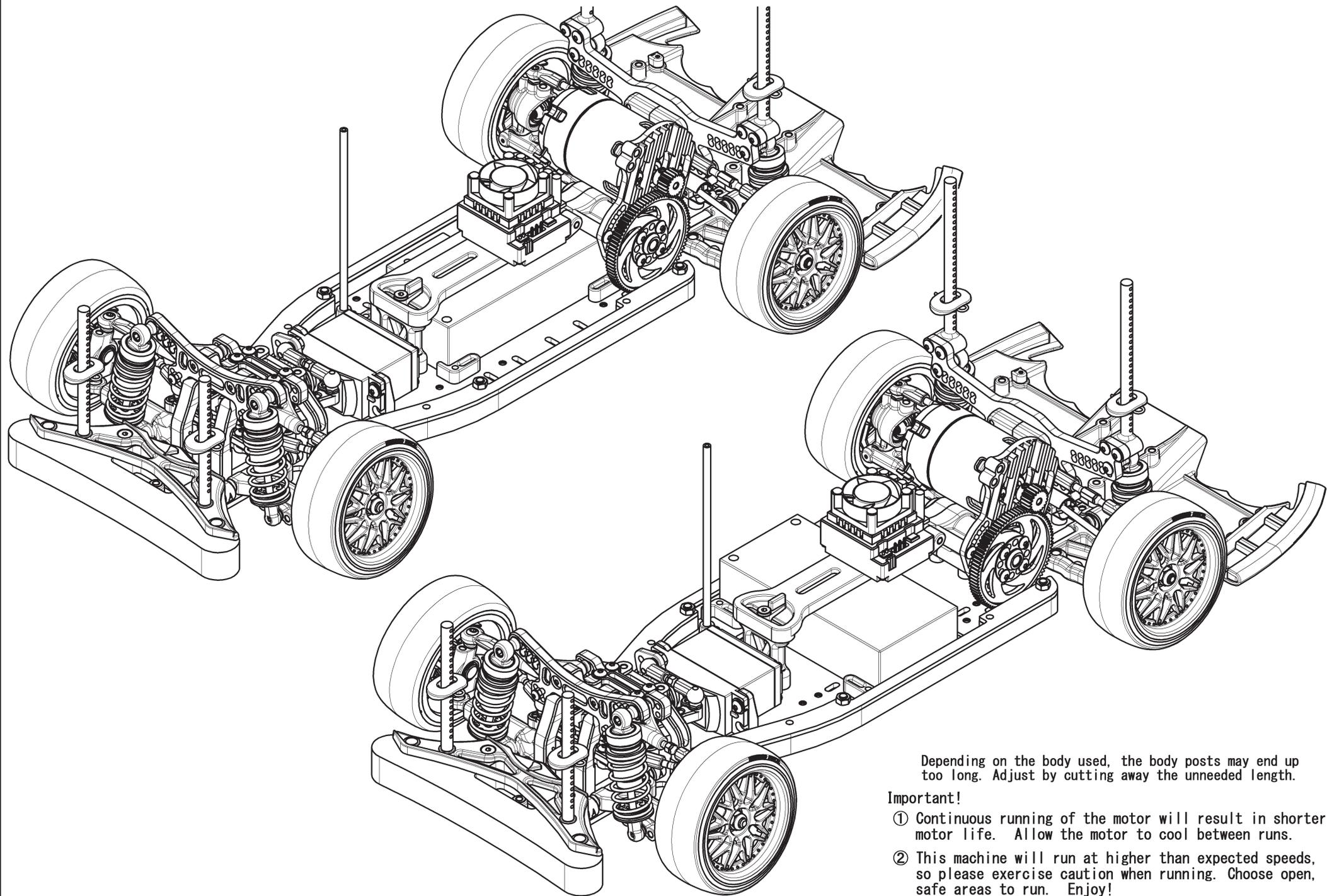
Depending on the body used, the body posts may end up too long. Adjust by cutting away the unneeded length.
