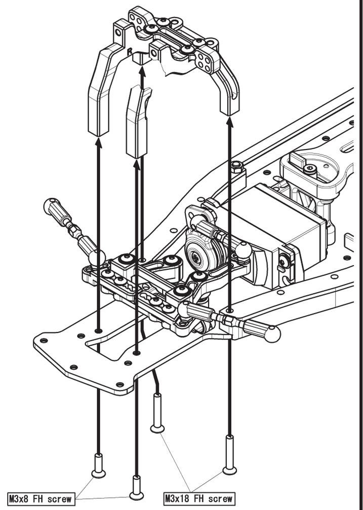
**Installing on front shock tower**
