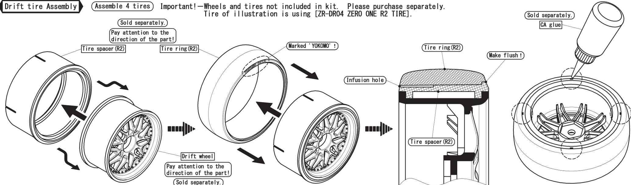
Install the tire spacer onto the wheel.
