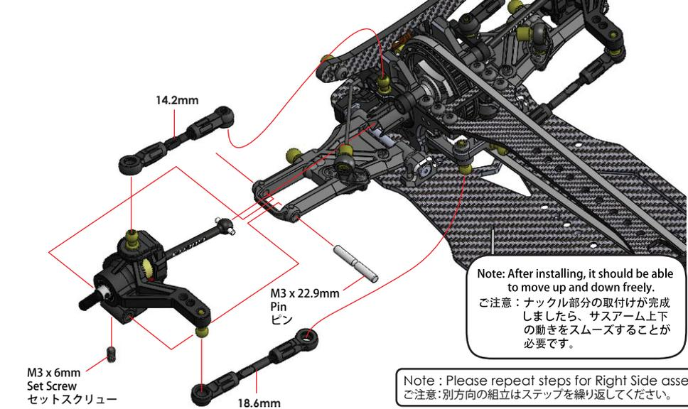
Note: After installing, it should be able to move up and down freely.
