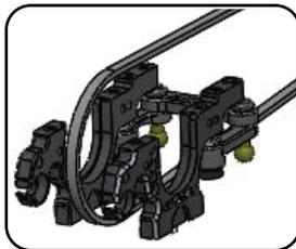
Note : Before assembly please put Midship Belt 423 between Bulkhead A & B to facilitate later drivetrain installation.
