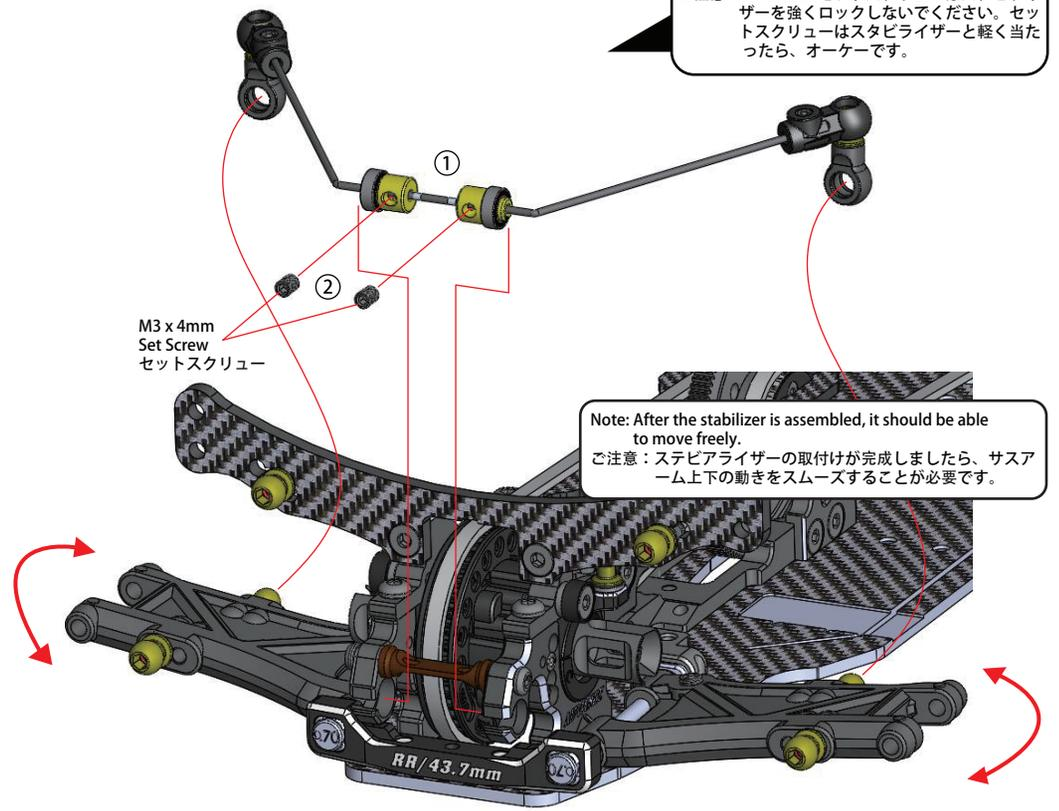
Note: M3 x 4mm Set Screw does not need to be tightened, just need to slightly touching the stabilizer.
