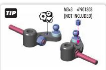
When using rearward hole, you can reinforce the steering block (for hard crashes) by installing an M3x3 setscrew in the forward hole.
