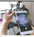
5. If the edge of the image is not sharp, loose the top knob to adjust the distance between the eyepiece and the camera. The distance will be different if you use different focal length eyepieces.
