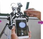
3. Put them on the telescope. Tighten the top knob of eyepiece clamp.
