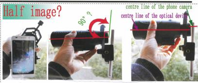
To get a whole image, you need to make the centre line of the phone camera and the centre line of the optical device coincide to each other.
