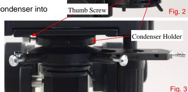
corresponding objective and annular ring must work together, i.e., **10X** phase contrast objective must work with **10X** condenser annular ring, and so on.
