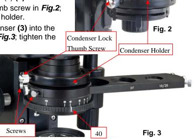
contrast objective must work with **40** condenser annular ring and iris diagram **40** (*Fig.3*) and so on.
