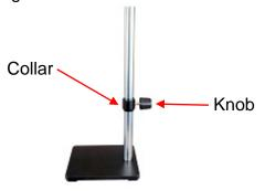
2.7 Slide the horizontal bar onto the pillar and stop at the collar. Then put back the cap on the top of the pillar.
