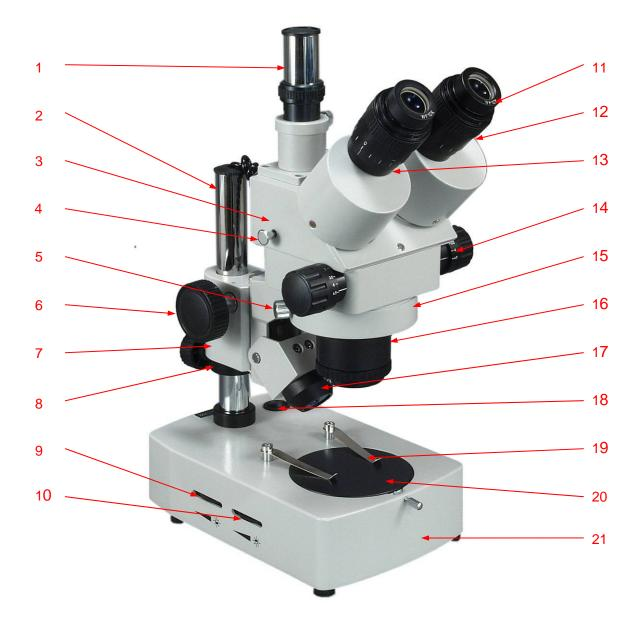
1 Photo Tube 8 Post Collar 15 Holding Ring Incident Light Intensity Dial Objective Housing Stand Post 2 9 16 10 Transmitted Light Intensity Dial 3 Trinocular Body Incident Light 17 Eyepiece/Photo Switch Eyepiece 4 18 Power Switch 11 12 Diopter Ring Stage Clip 5 Thumb Screw 19 6 Focus Knob 13 Eyepiece Tube 20 Stage Plate
