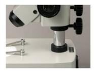
2.6.3 Slide the post collar to against the focus block as showed in the figure, and then tighten its knob.
