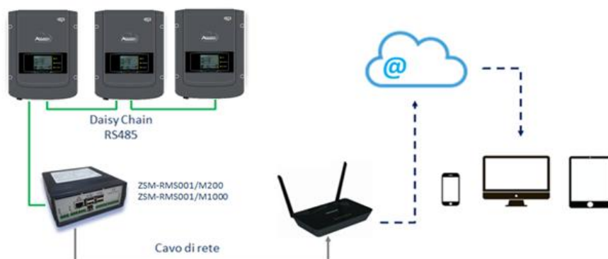
Figure 66 – Diagram showing the operation of the ZSM-RMS001/M200 / ZSM-RMS001/M1000 datalogger
