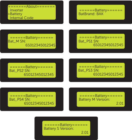
Figure 9-108 Displaying the battery information
