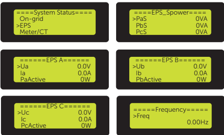
Figure 9-17 Displaying EPS status
