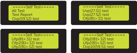
Figure 9-52 Setting to do tests
