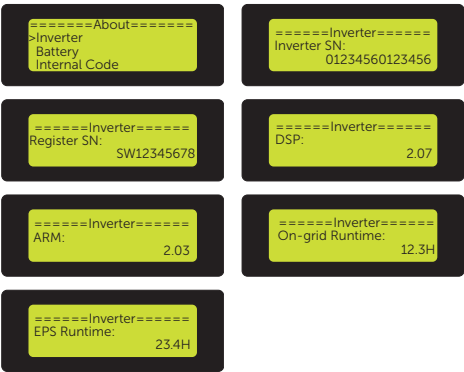
Figure 9-107 Displaying the inverter information
