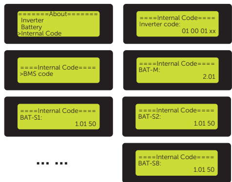
Figure 9-109 Displaying the internal code information
