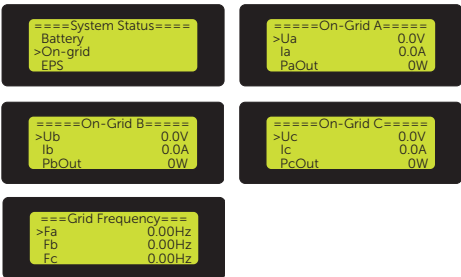
Figure 9-16 Displaying on-grid status
