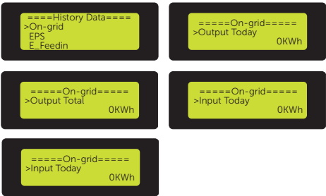
Figure 9-20 Displaying on-grid data
