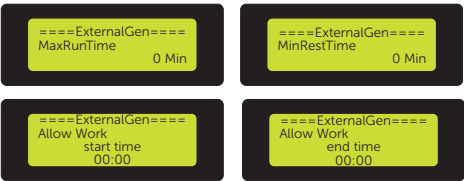
Figure 9-83 Setting MaxRunTime, MinRestTime, allow working period
