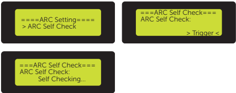
Figure 9-105 Triggering ARC Self Check
