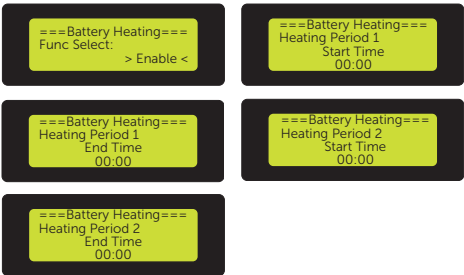
Figure 9-92 Enabling battery heating and setting working periods
