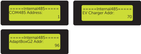
Figure 9-98 Setting the address of the external device
