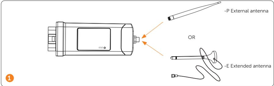
Step 2: Plug the Pocket WiFi into the correct port of inverter.
