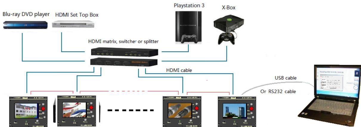
The DVM-HDT-KIT ANALYZER is an HDMI® sink emulator and can be used to test any HDMI® sources such as media players, BD players, switches, matrices, splitters, repeaters or literally any HDMI® device for proper functionality.
