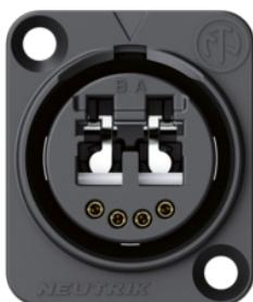
The chassis connector acts as a "feed-through" allowing simplified installations by connecting a conventional LC-Duplex on the rear. It is built in the standard D size shell and features an automatic sealing cover for maximum dust and dirt protection and a Push-Pull locking mechanism for safe connection.
