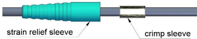
Slide the Strain Relief Sleeve and the Crimp Sleeve over the cable.
