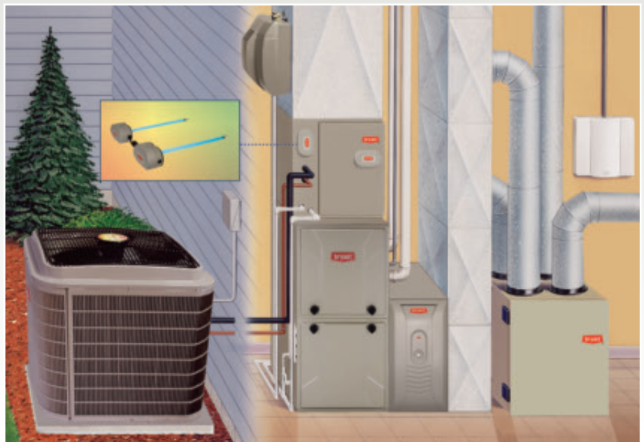
Air Conditioner and Gas Furnace System
