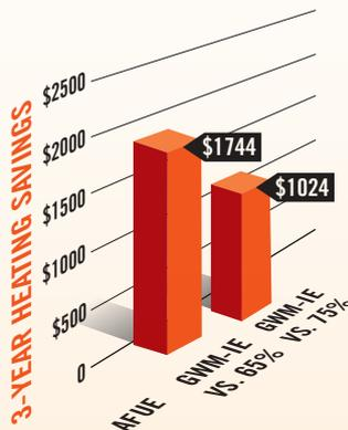
AFUE stands for "Annual Fuel Utilization Efficiency" and is a measure of a boiler's efficiency and performance. Like the miles-per-gallon rating on your car, the higher the AFUE rating, the lower your fuel costs. Typical boiler ratings range from 80% to 95%.
