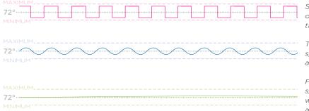
SINGLE-STAGE MOTOR: Since it's either full speed or completely off, a single-stage motor creates continuous temperature cycling throughout the day.
