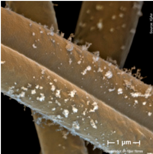
Diesel soot on Perfect 16 filter fibers. The tiny ultrafine soot particles are less than 1/10,000 of a millimeter.
