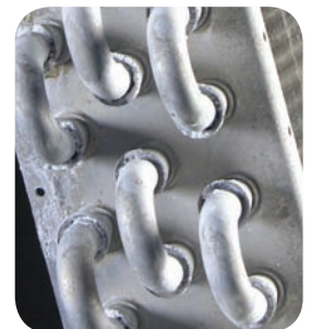
After 500 hours of salt spray, an all-aluminum tube sheet with an aluminum tube shows virtually no corrosion.
