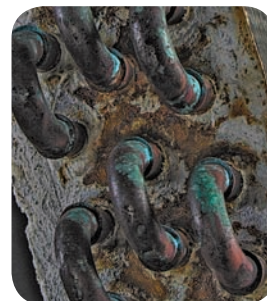
After 500 hours of salt spray, a galvanized steel tube sheet with a copper tube shows substantial corrosion.
