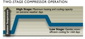
With its two-stage design, the 4SHP16LS makes the distinction between mild and extreme weather days, using only the energy necessary to keep you comfortable.
