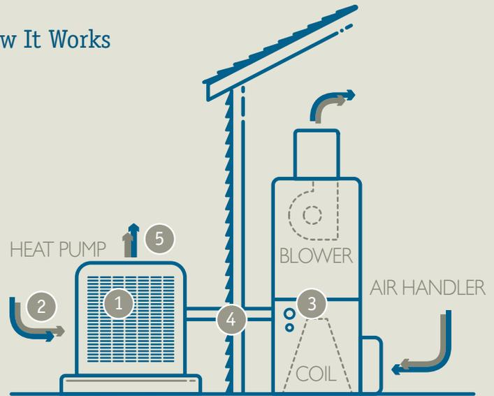
1. The heat pump on the outside of your home circulates refrigerant that absorbs and releases heat as it travels between the heat pump and the air handler inside.
