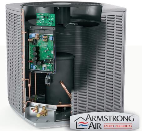
The 4SHP20LX variable-capacity heat pump helps keep your home's temperature precisely where you want it and may qualify for local utility rebates.\* Rather than running at one or even two speeds, the inverter-driven scroll compressor changes speed in small increments for exact temperatures. Plus Comfort Sync™ zoning delivers precise temperatures from room to room for complete home temperature control.
