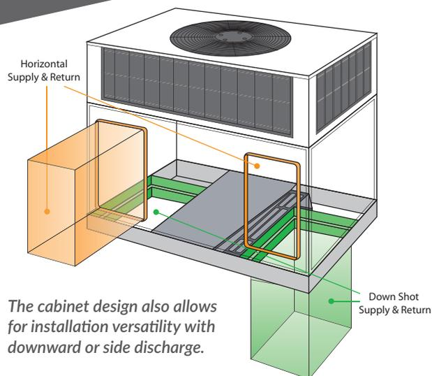
The cabinet design also allows for installation versatility with downward or side discharge.
