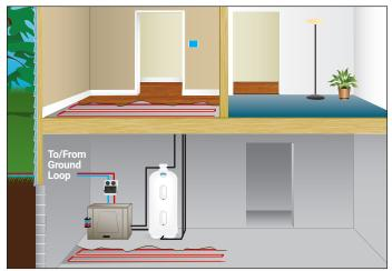
Common Water-to-Water geothermal installation
